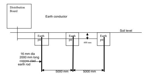
**Note**: The No. of earth rods shown is indicative only. These shall be increased until the desired Earth Resistance is obtained.
