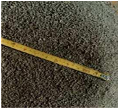
VSI Crushed Sand - Cubical - Good Quality
