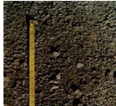
JAW Crushed Sand - Flaky - Poor Quality
