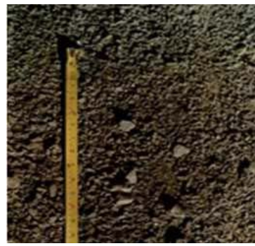
JAW Crushed Sand - Flaky - Poor
