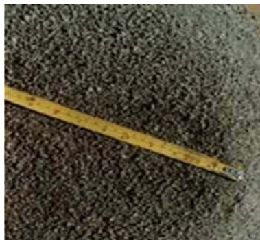
VSI Crushed Sand - Cubical - Good Quality
