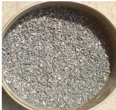
Poor Quality CS-Sand with Flaky Particles
