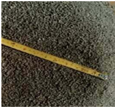
VSI Crushed Sand - Cubical - Good Quality
