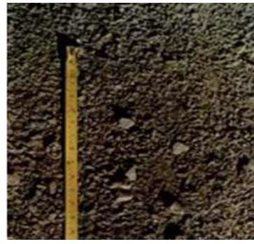
JAW Crushed Sand - Flaky - Poor
