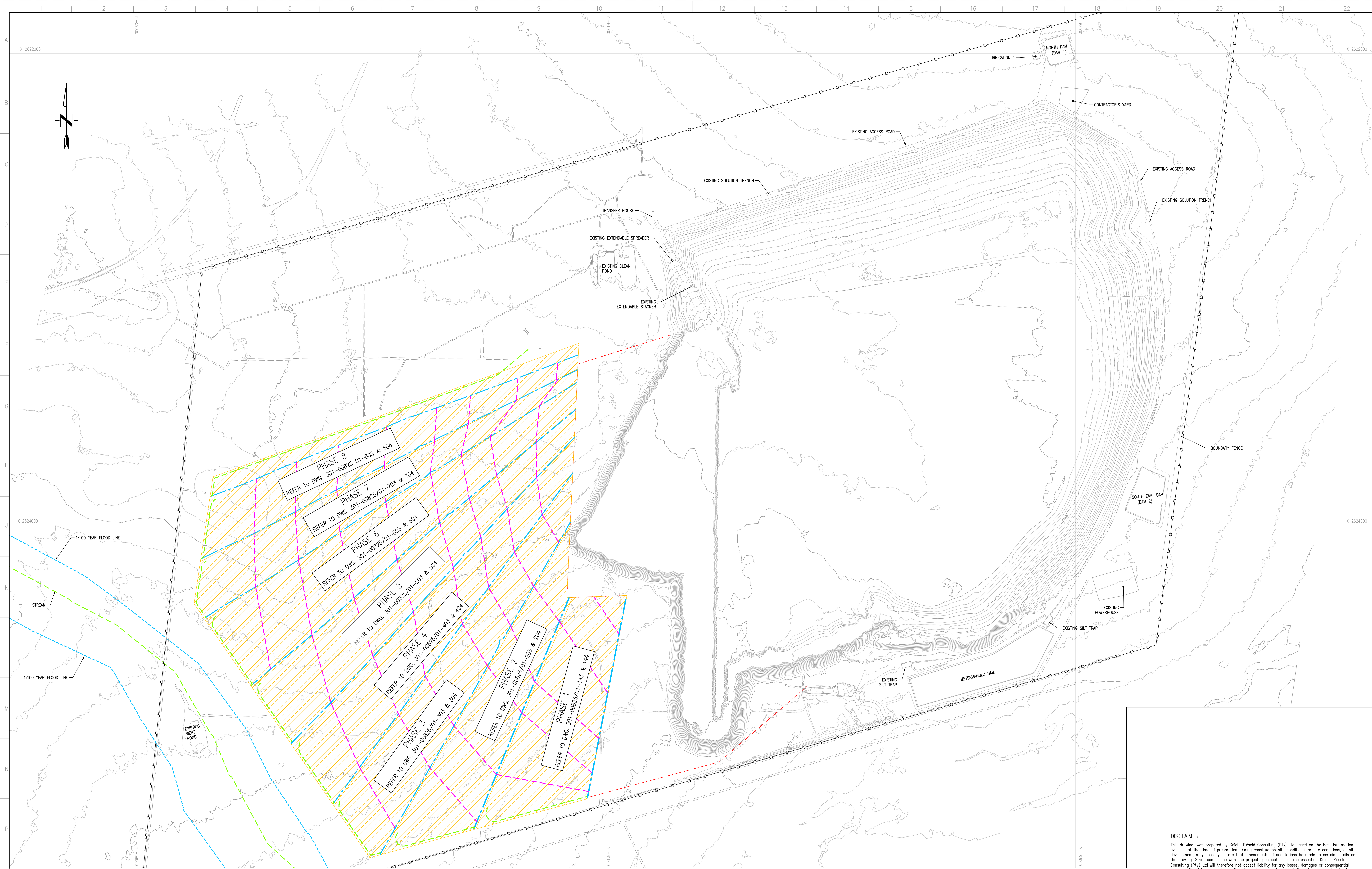
UNDERDRAINAGE LINER SYSTEM LAYOUT PLAN SCALE 1:5000
