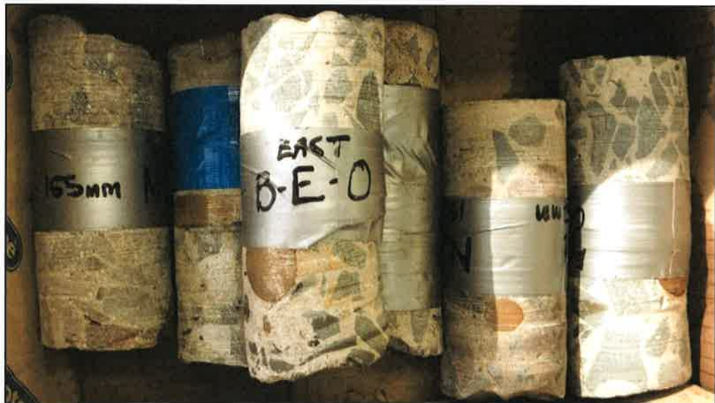
Figure 9: Concrete core samples retrieved from the berth's deck and piles
