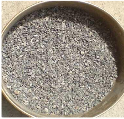
Poor Quality CS-Sand with Flaky Particles
