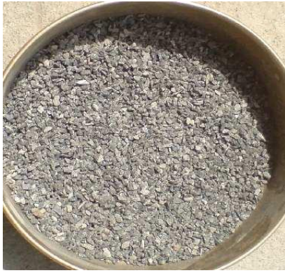
Poor Quality CS-Sand with Flaky Particles
