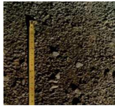
JAW Crushed Sand - Flaky - Poor Quality
