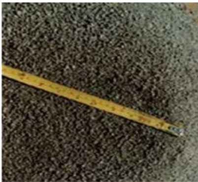
VSI Crushed Sand - Cubical - Good Quality
