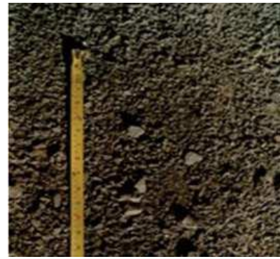
JAW Crushed Sand - Flaky - Poor Quality
