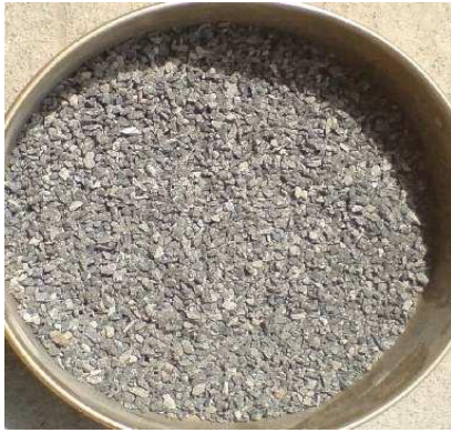
Poor Quality CS-Sand with Flaky Particles
