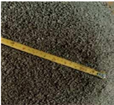
VSI Crushed Sand - Cubical - Good Quality
