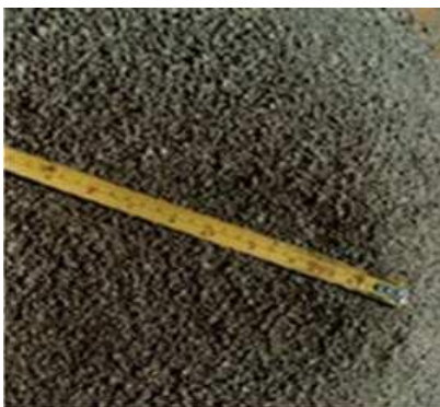
VSI Crushed Sand - Cubical - Good Quality
