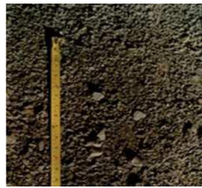
JAW Crushed Sand - Flaky - Poor Quality
