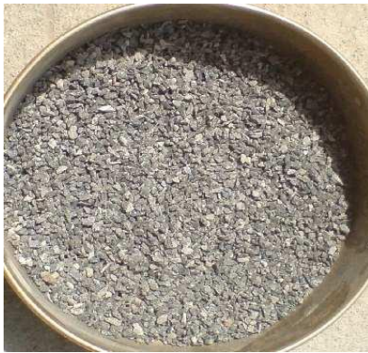
Poor Quality CS-Sand with Flaky Particles
