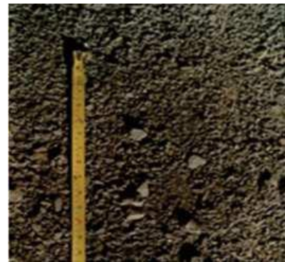
JAW Crushed Sand - Flaky - Poor Quality
