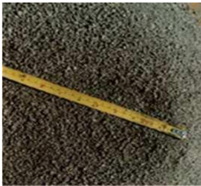
VSI Crushed Sand - Cubical - Good Quality
