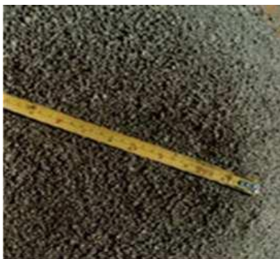
VSI Crushed Sand - Cubical - Good Quality
