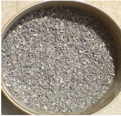
Poor Quality CS-Sand with Flaky Particles
