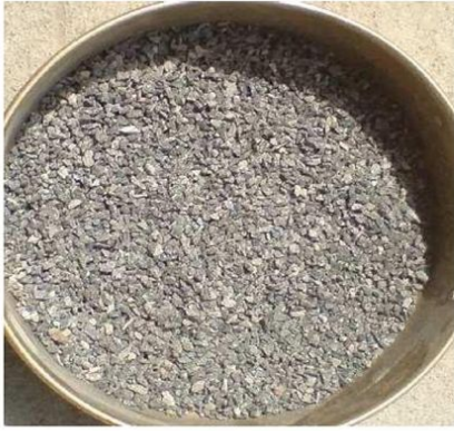
Poor Quality CS-Sand with Flaky Particles
