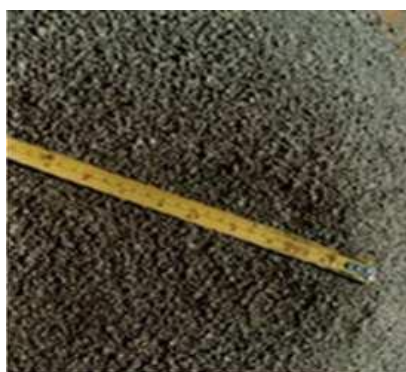
VSI Crushed Sand - Cubical - Good Quality
