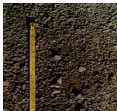
JAW Crushed Sand - Flaky - Poor Quality
