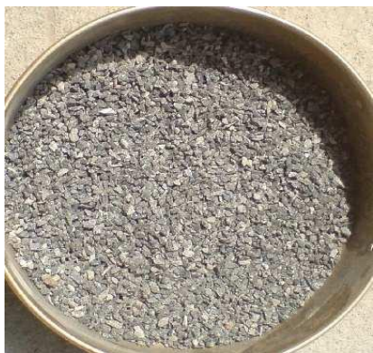
Poor Quality CS-Sand with Flaky Particles
