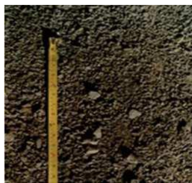
JAW Crushed Sand - Flaky - Poor Quality
