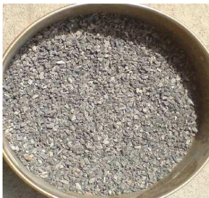
Poor Quality CS-Sand with Flaky Particles
