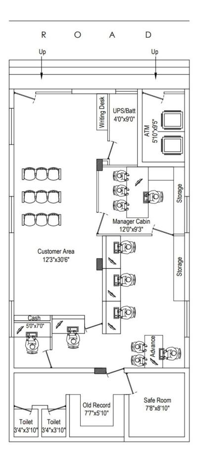
F8, 1st. FLOOR, BASCO COUR GANDHI BAZAR MAIN ROAL BASAVANAGUDI, BANGALORE G & G ASSOCIATES DATE :- 12 - 01 - 2022 SCALE :- 1" = 6'-5" ш GROUND FLOOR PLAN Option 2 TIME PROPOSED INTERIOR LAYOUT FOR UNION BANK OF INDIA AT KESTUR BRANCH. 30JECT >
